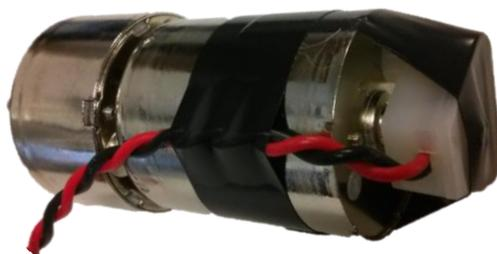
Figure 14: Securely fastened end cap.
