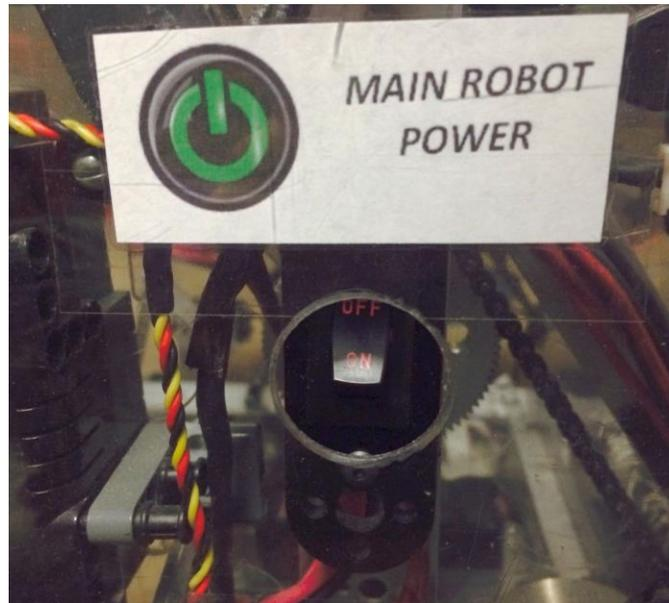
Figure 15: Power switch placement (behind plastic sheeting with an access hole).
