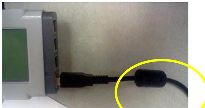
Figure 9: Ferrite choke in use on a USB cable
