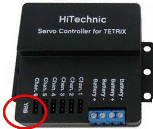
Figure 11: YRB Marking on the Servo Controller.
