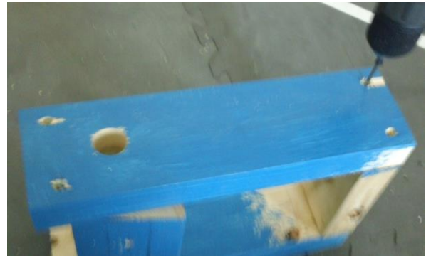
Step 1-6: Fastening the other 2x4x12" board to the bottom 2x4x5.5" board.
