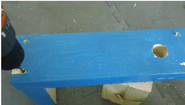
Step 1-4: Fastening the bottom 2x4x5.5" board to the 2x4x12" board using 3" wood screws.
