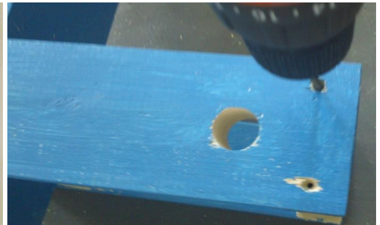
Step 1-11: Fastening the 2x4x5.5" board (W5) to the top of the 2x4x12" boards, after the boards have been made flush to one another.
