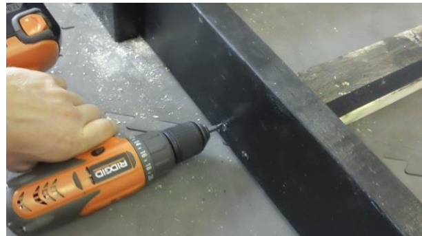
Step 3-8: Replace the crossbeam in the correct position and use two 2" 10-32 machine screws to secure the crossbeams to the sidewalls.
