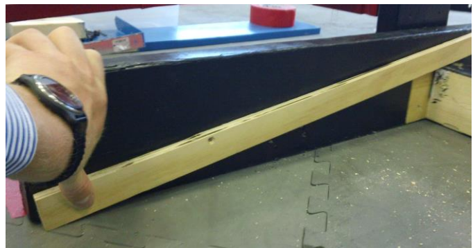
Step 3-2: Trace a line on the sidewall for guidance from the top of the center crossbeam, to the bottom edge of the sidewall, stopping at the mark 0.375" in from the outer edge.
