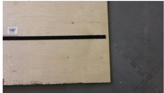
Step 4-5: Place a Velcro strip (loop side) along the mark.
