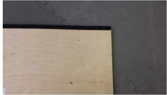
Step 4-3: Place a strip of Velcro (loop side) along the edge of one of the 2'x4' panels (W7). This strip will match up with the hook side strip on the center crossbeam.
