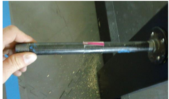
Screw the two 10" balance arm support tubes into the pipe flanges located on the vertical 2x6's.
