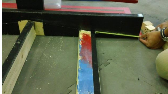
Step 4-2: Measure the distance from the edge of the sidewall to the Velcro strip on one of the outer crossbeams.
