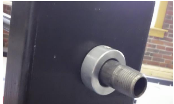
Align the pipe so it sticks roughly 3" out from the vertical arm and place a collar flush against the outside of each vertical arm. Tighten the set screw to secure the collar in place.
