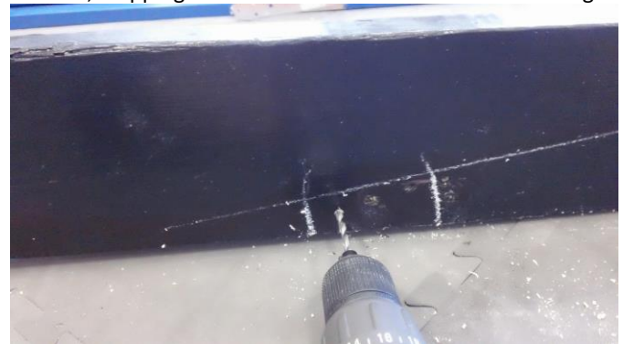
Step 3-4: Drill two evenly spaced pilot holes through the crossbeam, within the confines from the traced 2x4 using a 13/64" drill bit.
