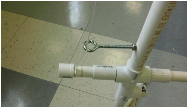
Thread line through bottom eyelet and hole drilled in shaft. Secure with double knot.
