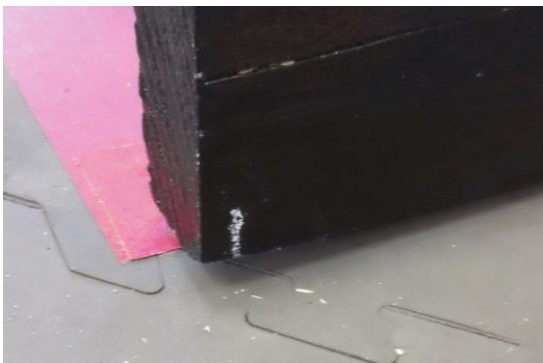
Step 3-1: Make a mark 0.375" in from the outer edge of the sidewall.
