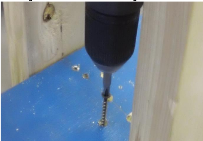
Step 1-10: Fastening the 1x6x48" board (W4) to the 2x4x5.5" board (W5) using 1.5" wood screws.
