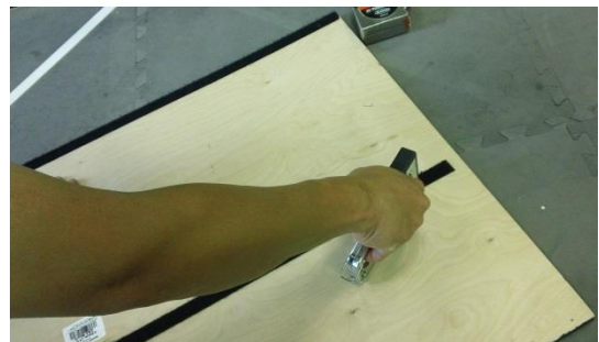
Step 4-7: Secure the Velcro strips with staples, and then repeat the process for the other 2'x4' board (W7).
